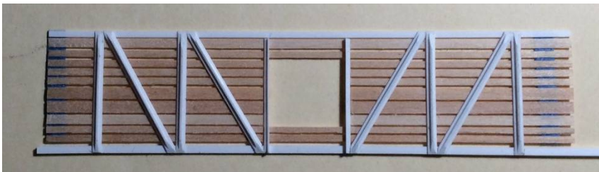
Photo 9 Side 1 with all vertical and diagonal braces installed
