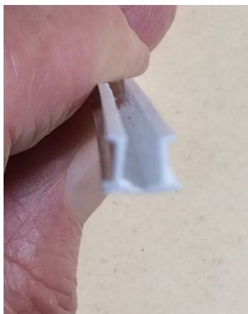
Photo 14 Center Sill I-beams with inner top flange of I-beam removed
