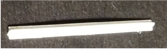
Photo 7 Back to back pieces of Plastruct 3/64" angle glued together to create one of twenty four braces
