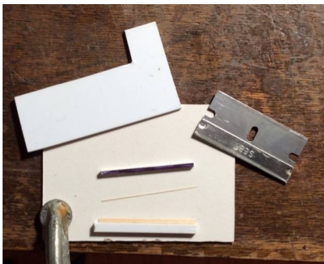
Photo 4 Tool/jig used to cut a piece of NSL 1"x 6" lumber down to 1"x 5.25". The sliver that was cut off can be seen in the photo.
