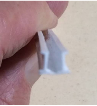
Photo 5 Center Sill I-beams with inner top flange of each I-beam removed
